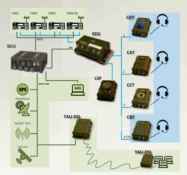
A **DCU** is the central control switchboard and gateway into the external environment, which allows the creation of MANET mobile ad-hoc dynamic networks on narrowband radio networks.
